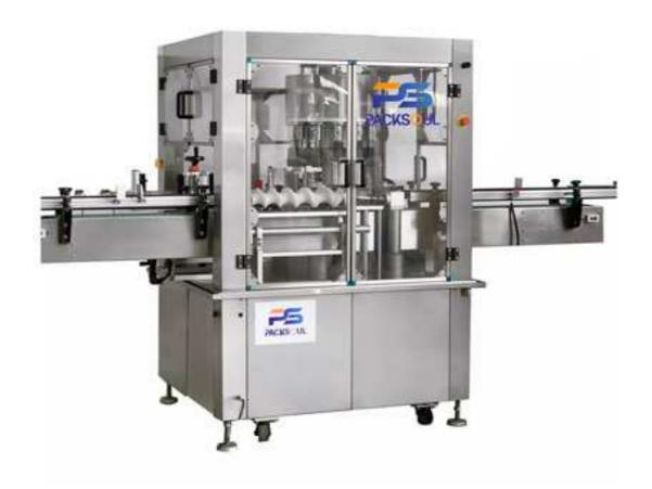
PACKSOUL rotary type sticker labeling machine is for high speed capacity sticker labeling and for the products what need locate the label position. Compare with linear type, the rotary type can meet the high capacity requirement and can solve special labeling requirement such as sticker positioning, multi-sticker labeling etc.
