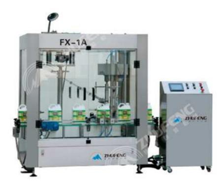
This machine is protective automatic capping machine and control by PLC program. Bottles will be fixed by two cylinders and it can automatically arrange lid, taking lid and sending lid, it will first grasp lid then capping under control of double-acting cylinder lifting stroke. The machine grasp lids through pneumatic type, lid-revolving head has a clutch to ensure the tightened lid not to damage. It suits for capping of 5-10kg drum plastic large diameter caps.
