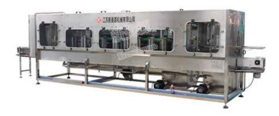
The machine is used to brush the outside of 5 gallon bottle, and then washed by pure water.
