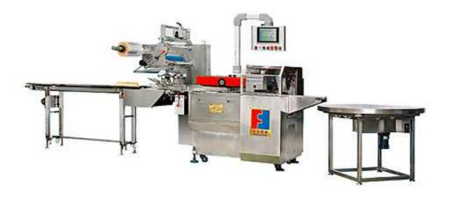
FFA-MA adopt full servo motor control to achieve conveyor feeding. This machine do not need pusher, the photo cell will inspect the product length and adjust the sealer automatically achieve full automatic packing. So the machine can pack different sizes of product do not need to change anything.
