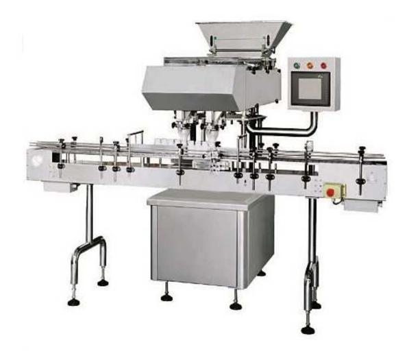
Fully automatic bottle filings machine, max speed is up to 6000~12000 tablets/min
