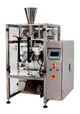
Vertical full automatic sauce filling machine can freely adjust the filling volume and filling speed with high filling accuracy. The contacting material part is made of 316 stainless steel. Filling bulkhead with anti-drip and upgrade filling device; complete automatic feeding, metering, filling Bag, date printing, the product output all the production process. It is easy to operate and maintain.
