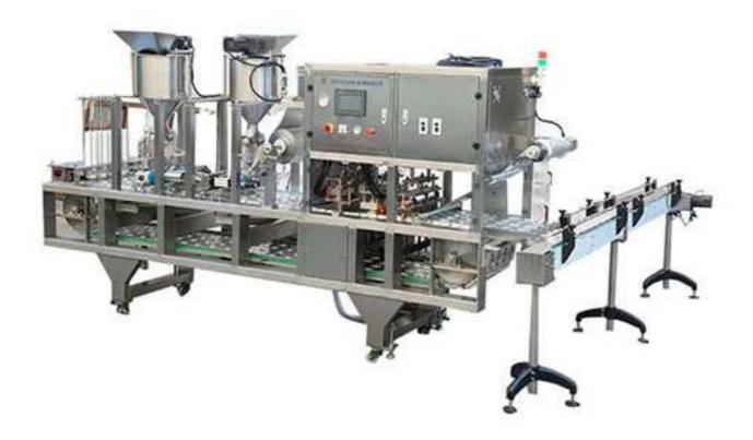
Cup filling and sealing machine have different specification sealing pump. We can design different machines as per client's requirements. It is suitable for filling and sealing any level drink and pasty products in different shapes and capability vessels. For example drink, water, milk, yogurt and so on.
