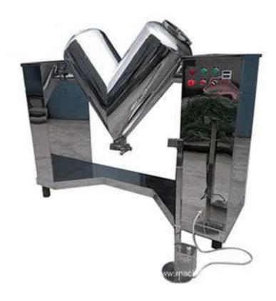
V Mixer Machine is applied to good liquidity dry powder and granular material mixing from many industries. This Mixing Machine has a special structure, its mixing efficiency is high and no blind corner. The machine is made of 304 stainless steel, 316 stainless steel can be customized as required. And the mixing barrel is polished both inside and outside. The material in the V-type mixing container flows smoothly without damaging the original material.
