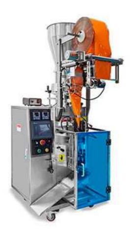
The Granule Sugar Salt Snack Packing Machine is suitable for food processing industry. This machine integrates automatic weighing, bag making, filling, sealing, automatic built-in label, printing and counting. Touch screen control, man-machine relationship is more good, the operation and use are very convenient. Its packaging speed can reach 30~80 bags/min, which can greatly save time and cost.
