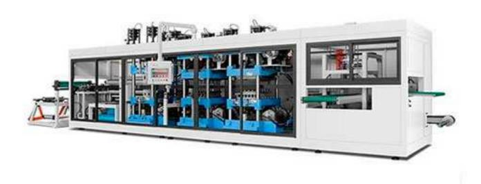
Fully automatic disposable food container making machine is our latest developed core product. The machine combines forming, punching, cutting, and stacking into process. widely used and suitable for most of the customer requested, it can produce plastic trays, containers, boxes, lids, etc. The machine is completely driven by servo motor, stable operation, low noise, high efficiency, high quality.
