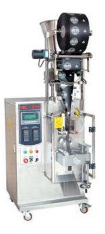
The MK-60KZ Vertical form fill seal machine automatically performs bag forming, filling the bag with product, weighing, sealing, bag cutting, counting, code printing, finished package discharging, etc. Using s measuring glass for weighing, this packaging machine suits the wrapping of uniform, loose, non-viscous, fine granules.
