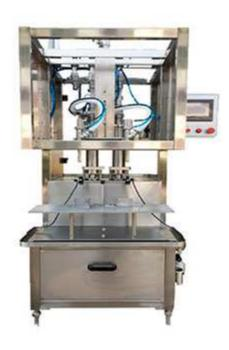
This machine is suitable for filling water and cream products, especially for high viscosity materials (such as daily chemical, washing chemical, suspension agent, etc.). Equipped with touch screen man-machine interface system; Manual bottle feeding, automatic filling and manual bottle discharging; Servo motor drive, ball screw drive, control the movement of piston rod to ensure the stability of filling; The machine conforms to GMP requirements.
