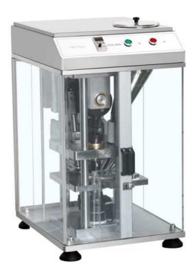
This machine is a continuous automatic tablet press designed using advanced foreign technology and used in medicine, chemical industry, electronics, food industry to press powder and granular raw materials into tablets.
