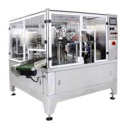
ZH-GD8 Rotary packing machine is developed for premade pouch, stand-up pouch with or without zipper. It is suitable for packing product of powder, irregular shape, thick liquid and liquid, such as gourmet powder, chicken powder, seasoning powder, candy, fruits, nut, pet food, roasted seeds, puffed food, frozen food, small hardware and hand sanitizer.
