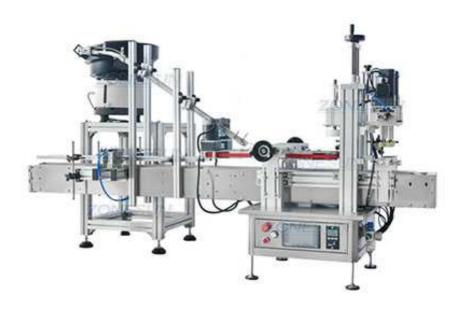
This automatic capping machine is good for various bottles like spray bottles, dropper bottles, trigger pump bottles. It is designed with bottle guiding structure, this is good for bottles that are easy to fall down during capping work, it can improve production quality. This machine is widely used in food, cosmetics, daily chemical industries.
