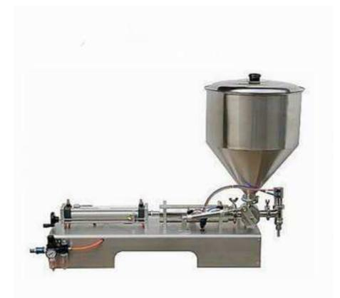
DG semi-automatic piston single head filling machine is the company's development of DTG semiautomatic piston filling series of a kind of the high concentration of fluid filling machine, it is through the cylinder, a piston and rotary valve tee to extract and with high concentration of material, principle and air cylinder is controlled by magnetic reed switch trip, you can adjust the filling quantity.
