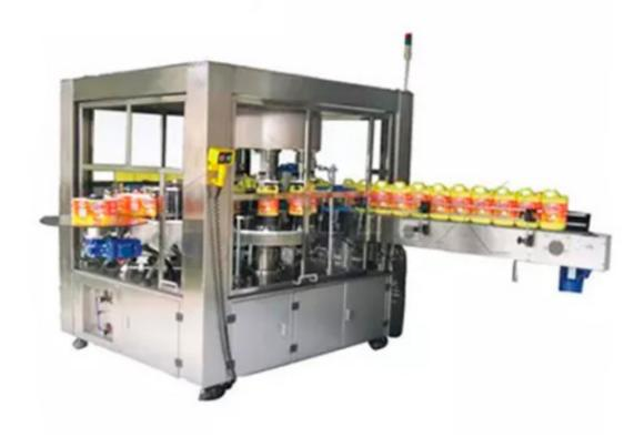
Hot melt adhesive labeling machine: suitable for round bottles, square bottles, flat bottles, oval and other PET and glass bottles or containers. It is suitable for labeling before and after filling. It has the characteristics of reasonable design, reliable performance, low operating cost and high cost performance.
