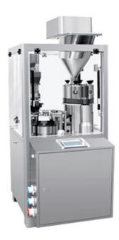
NJP-200A Fully Automatic Capsule Filling Machine is filled by powder, grain, and tablet. It adopts multi-bore dosing, intermittent motion and timing frequency conversion. It is suitable for automatically completing capsule feeding, separating, filling, (waste capsule rejecting), closing, finished product ejecting for powder or tiny pill medicine in capsule. It is designed sophisticatedly by our factory according to the practice on domestic; it is fully accord with the GMP standard.
