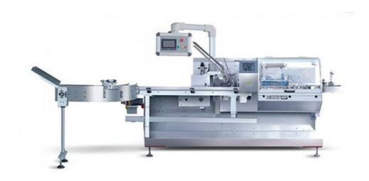
ZHW-120 Automatic cartoning machine is widely applied in ice creams, tubes, soap and other similar objects cartoning packing. The machine can automatically finish filling packaged, forming carton, inserting packaged objects, embossing batch No., close carton and finished product output functions.
