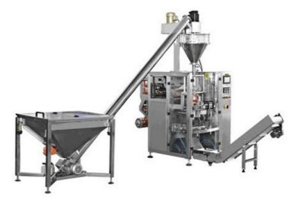
Automatic vertical powder packing machine is specially designed for packing powder material within 100 meshes. The vertical packaging machine unit adopts screw elevator system and auger weighed system which focus on powder material elevating and weighing. Presently, The vertical form fill seal machine unit is widely applied in Grain Powder / Food Additives / Milk Powder / Cereal Powder Or Similar Material.
