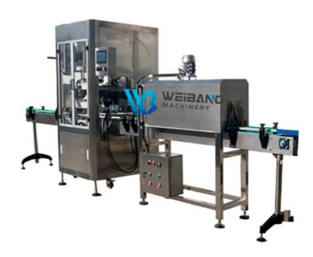
Automatic band shrink wrap machine hemp essential oil bottle shrink sleeve labeling machine, PLC control system, touch screen display and trichromatic lamp alarm prompt, timely find out equipment failure reasons.
