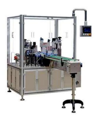
This machine is used for filling mascara, lip gloss, foundation liquid and other cosmetic products. It adopts cam type quantitative filling, tank is designed with pressuring system for mascara product, easy to operate and clean.
