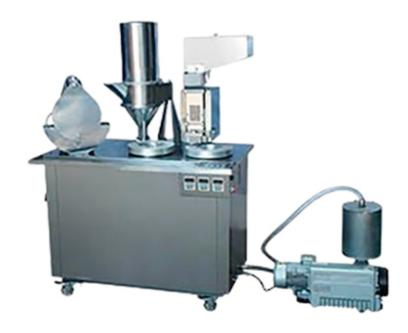
Integrating machine, electricity and air, the machine is easy to make separate operation of such actions as feeding, separation, filling and locking etc. The machine and working panel are made of stainless steel, which conforms to sanitary requirements of pharmacy. It is also suitable for filling powder of granular medicines and health products into capsule.
