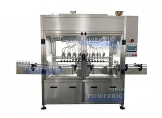
A deodorant filling machine is a type of machinery that is specifically designed for filling deodorants into containers, such as spray cans, roll-on bottles, or stick containers. This machine automates the filling process, which helps to improve the efficiency of the production line and reduce the likelihood of errors or inconsistencies in the amount of deodorant being filled into each container.
