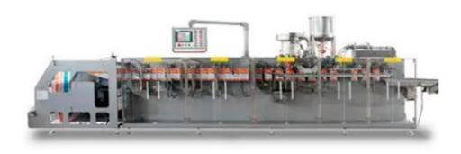
DZS-280 series Automatic Horizontal Doypack Packaging Machine has doypack function &duplex design, meet multifunctional packaging requirement like hanging hole, special shape, zipper or spout, the filling capacity is 600ml, the maximum speed can reach 120bags/min.
