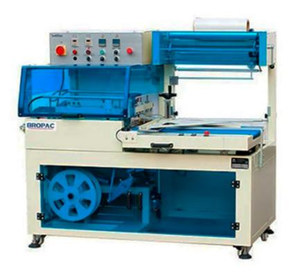
FQL450LB automatic L-type sealing machine concentrates bag-molding, sealing, cutting and object transmission in one operation; use shrink film as packaging materials. It has advantages of simple operation and high capacity. It is suitable for the need of big scale production.
