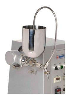
Homogenizer unit is suitable for mixing of different types of liquids like oil in water & water in oil construction up to 30 kgs. / Hour. A piston pump produces homogenization. Materials can be filling to pump from a hopper, having a capacity of 1.5 litres.
