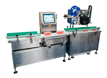
The equipment is an automatic weighing printing and labeling machine; the product is connected to the automatic weighing machine, and the weight information is sent to the instant printing and labeling machine in real-time;
