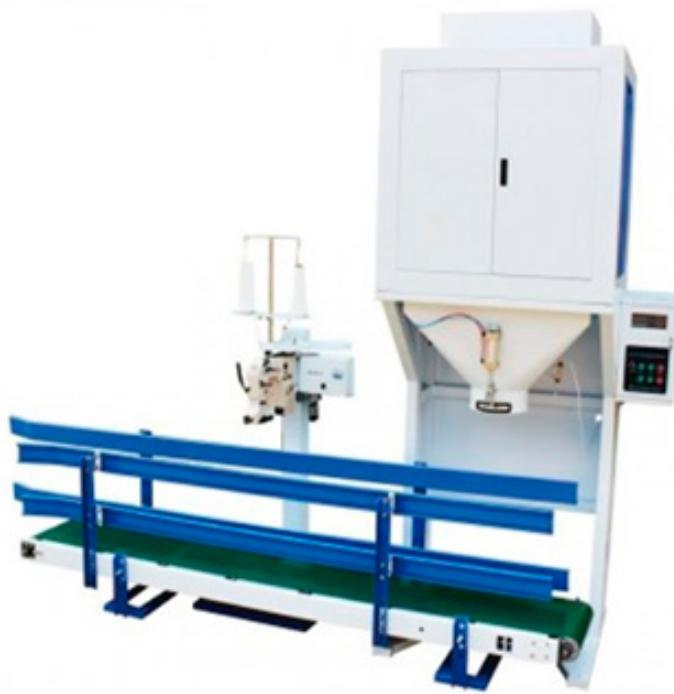
The total unit includes one set of CJS system automatic weighing machine, one set 2.5 meters belt conveyor, one set of sewing machine, used for weighing filling granules, such as: rice, seeds, grains, etc. in pp woven bags and sewing the bag.
