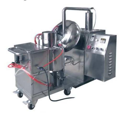
The machine is used to carry out sugar coating and film coating the core of Chinese traditional medicine and western medicine tablets, it integrates strong power, weak power and hydraulic pressure with pneumatic operation, it is new type equipment improved on the basis of original common type sugar coating machine.
