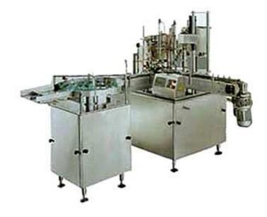
The eye drop filling is mainly made up of bottle setting machine, two-head filling machine, fixing inside lid, outside lid and revolving lid, implicated in the dropping of the fluid eye plastic bottle, glass bottle and mould bottle.
