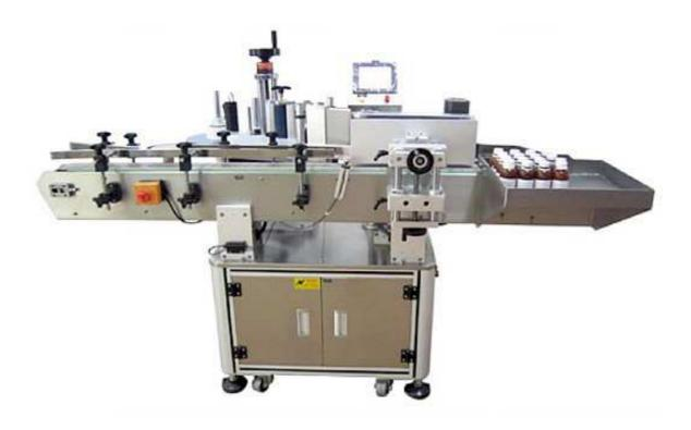
It adopts vertical type transmission, vertical type labeling, more stable, and more precise and improves working efficiency.
