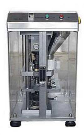
DP-12 Single punch laboratory tablet press machines are developed after the absorption of foreign advanced technologies. They are the automatic laboratory tablet press machines to press powder and granular substance into tablets continuously used by departments such as pharmacy, chemical industry, electronics, foods and laboratories.
