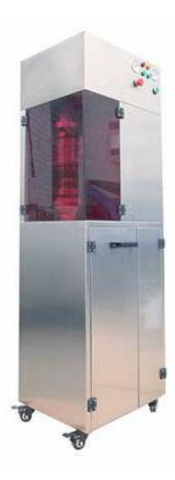
In the relatively airtight environment-working cabin, use high and low pressures to alternate changes rapidly "pressure shear" causing pulsed drawing force to the capsule. Under the continuous function of the pulsed drawing force, the capsule is gradually drawn and separated.
