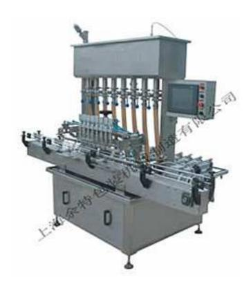
The CGF series injection filler is a high-tech product designed and developed by our company. It mat suit for different viscosity of water agent, semi-fluid and paste, it is widely used in the product filling of foodstuff, cosmetics, medicine, grease, daily chemical industry, detergent, pesticide and chemical industry. Using the straight filling way, may be used in the different vessels, needn't add any parts.
