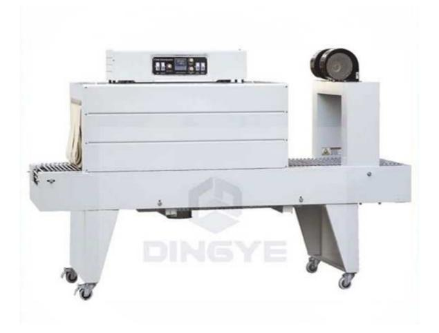
The BSE series PE film shrink tunnel is suitable for all kinds of shrink films. The machine adopts digital temperature controller, which makes operation easier. There are shrinking tubes on the top, bottom and sides of the shrinking room. The powerful fan inside the tunnel makes the air heating equally. The speed of the conveyer is adjustable. And you can choose roller or net conveyor as your request.
