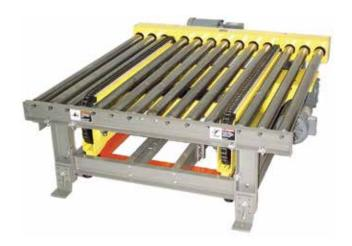
Premier Tech Chronos chain transfers are used to move unit loads on and off the CDLR conveyor at right angles to the direction of travel. The transfer is contained inside a welded structural channel frame. A pneumatic wedge lift mechanism which raises and lowers the chain transportation conveyor through the roller spacing in the companion CDLR section. Optional pop-up load stops can be added for squaring loads and guaranteeing pallet positioning prior to transferring the pallet load.
