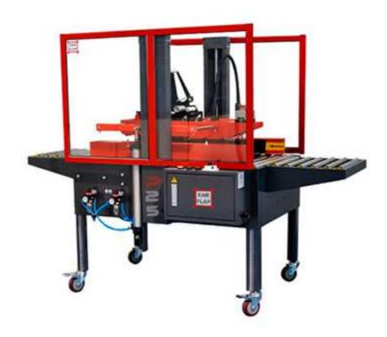
The Model P25 Carton Sealer is a small, multi format, carton sealing machine from Spanish manufacturer Ear-Flap that is capable of taping cartons up to 480mm in width and 480mm in height. It can tape both the top and bottom of a carton and has automatic adjustment for carton width and height.
