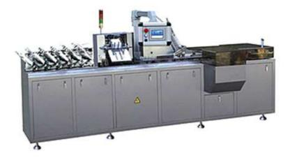
This machine is suitable for sachet, pouch, soft al/al strips, wound plaster, ointment plaster, facial mask plaster, coffee bag into carton. On line product feeding and detecting, leaflet fold (I-4folds) and feeding, leaflet detecting, canton opening and forming, products and leaflet pushing into carton, printing batch number, sealing carton with tuck-in or hot melt glue device. Automatically reject lacking of leaflet or product and finished product out.
