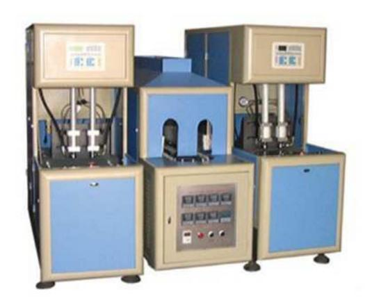
Semiautomatic bottle blow molding machine is suitable for producing PET plastic containers and bottles from 0.1L to 2L. It is widely used to produce the carbonated bottle, mineral water bottle, pesticide bottle, oil bottle, cosmetics bottle, wide-mouth bottle etc.
