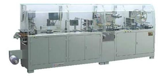
DPR-250B Tropical (ALU-PVC-ALU) Blister Packaging Machine is the innovation product in China and got two patents of the state. It can be used for three packing kinds for ALU/PVC, ALU/ALU, ALU/PVC/AVC and up to the purpose that a machine with three usages just to change moulds.
