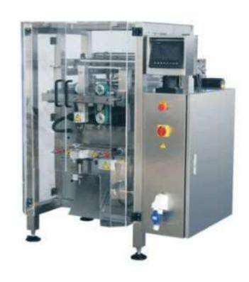
Automatic Vertical form-fill-seal packing machine explores the roll of film to make bags of pillow bags, gusseted bags. The maximum film width is 240mm. Small loading weigher can be added which is up to 200g. It can automatically realize bag making, filling, printing, sealing, gusset making, hand hole making, etc.
