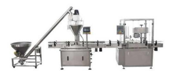
This is a fully automatic tins and cans filling sealing packaging line, which is applicable for packing different products, such as coffee powder, coffee beans, chocolate powder, tea, nuts, olive, dairy product, oil, drinks, etc. This machine is suitable for all kinds of tinplate cans, aluminum cans, plastic cans and paper cans. The machine is easy to operate with high quality.
