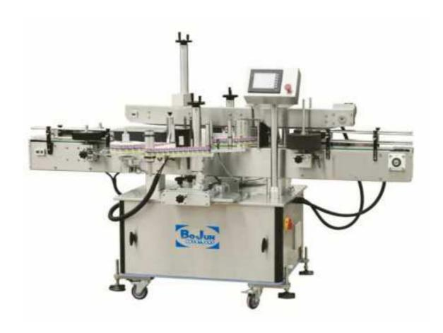
This machine is suitable for automatic double-sided labeling of flat, square and round bottle products. The use of double-sided chain correction device to ensure that the bottle of the neutral; special flexible pressure device to ensure the stability of the bottle.
