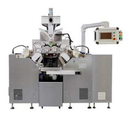
RGY12-15 IV softgel encapsulator is the most advanced soft capsule production equipment. The equipment has an all-servo control system, which provides greater output and stable performance, enabling more automated production.
