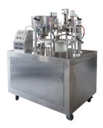
The NF-10 plastic and tube filling sealing machine is mainly used in a transmission principle. Dividing mechanism drive with a fixture of the rotary table is used as the intermittent movement, complete interior, and exterior heating, automatic filling and sealing, pressure, trimming, finished product exit and a series of functions.
