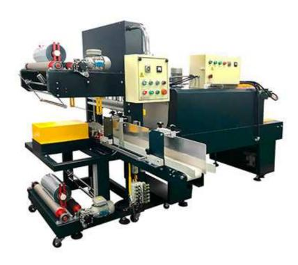
Sleeve-type Sealer with Tray Model, SSA600U / SSA800U has automatic operation of feeding, pushing & sealing to work with heat tunnel, especially it can run PE or PVC for big size carton, multiple package & package with tray for shrink pack; furthermore, machine can be worked either inline or off-line automatically.
