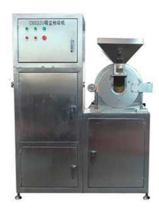
The grinder set consists of grinder, EXC collector of raw material and ESC collective duster. It solves the problem, i.e. the dust is flying during the period of crushing raw material.
