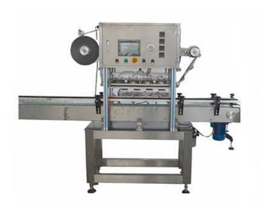
The automatic aluminum foil sealing machine is based on the principle of electromagnetic induction. The aluminum foil on the bottle mouth generates high temperature instantly, and then the aluminum foil is fused on the bottle mouth to achieve the sealing function. It has good moisture-proof, mildew proof and anti-counterfeiting functions, thus prolonging the storage time of articles.
