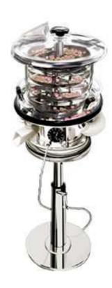
Model C&C200A Tablet Deduster is suitable for the deduct of any type of tablets. The whole operation process can be monitored. Between each of the sieve discs the separation part can effectively sep-arate the tablets and powder. It is adapted to any types of tableting machines.
